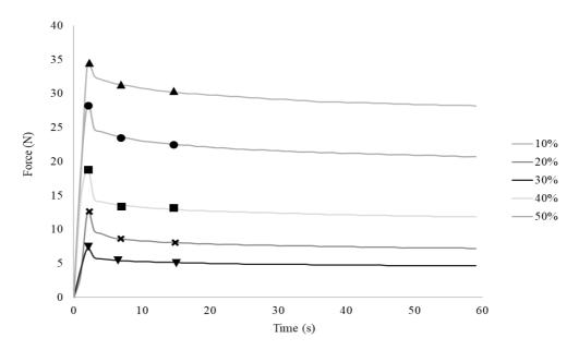
**Figure 4** The hardness test results with variations in the composition of rice adhesives.
