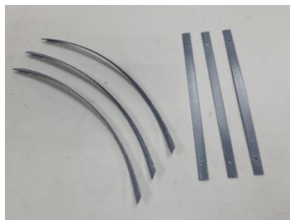
Figure 9. Helical NACA 0015 blades (Left) and Straight NACA 0015 blades (Right)
