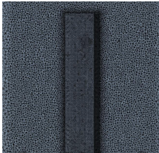
Figure 7. Mesh refinement applied on the building.
