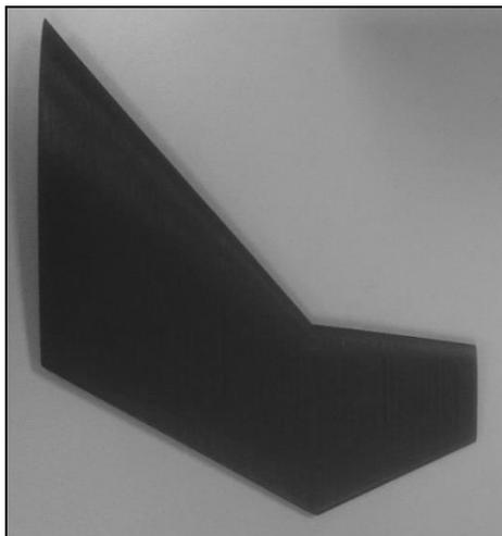
**Fig. 3.** 3D printed cranked wing.
