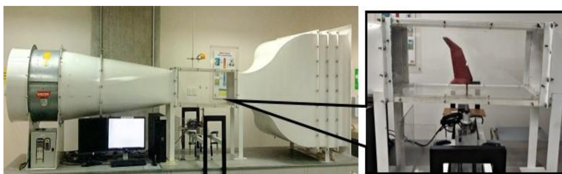
Figure 3. TUWT (Left) and Test Model Installation Method (Right)
