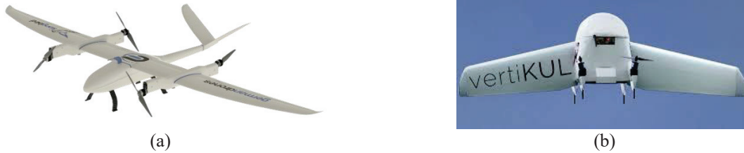
FIGURE 2. (a) Tilt-rotor convertiplane [10]. (b) Tail-sitter [11].
