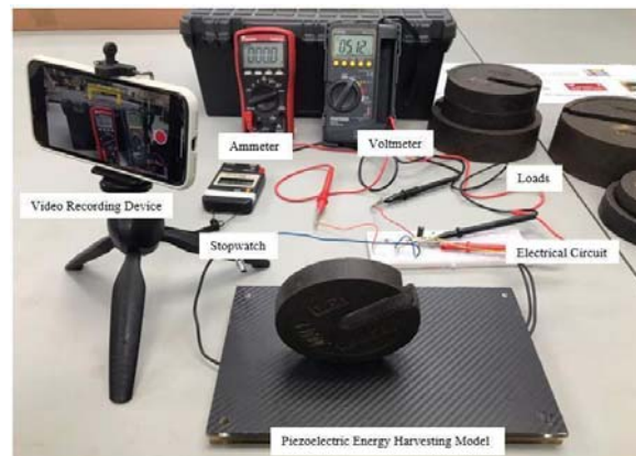
Figure 8. Experimental setup for piezoelectric energy harvesting system.
