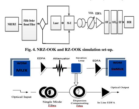
Fig. 5. Transmission link set-up.
