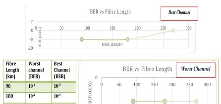
Fig. 10. BER values for 4 Channel WDM RZ-OOK (Bit Rate~ 40 Gb/s).
