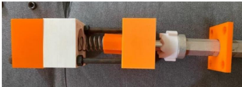
Figure 8. Unassembled exploded view of the prototype leg unit assembly
