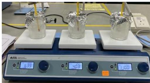
*Fig. 1. Experiment set-up for blood mimicking fluid formulation*
