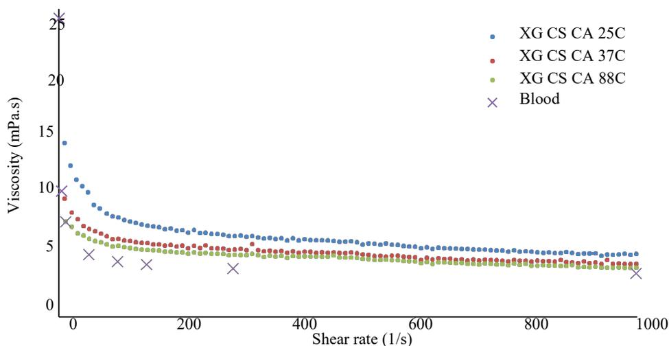
Fig. 2. Viscosity against shear rate for xanthan gum-corn starch-water glycerol base and contrast agent with variation of mixing temperature.
