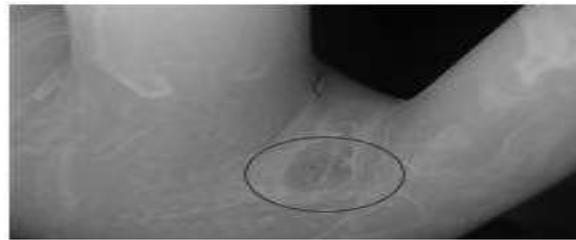
Figure 1: ‘Fisheye’ defect located in powdered glove.
