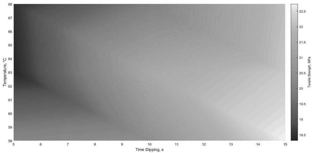
Figure 9: Contour of temperature and time against tensile strength of glove for 0.03 wt% of wetting agent
