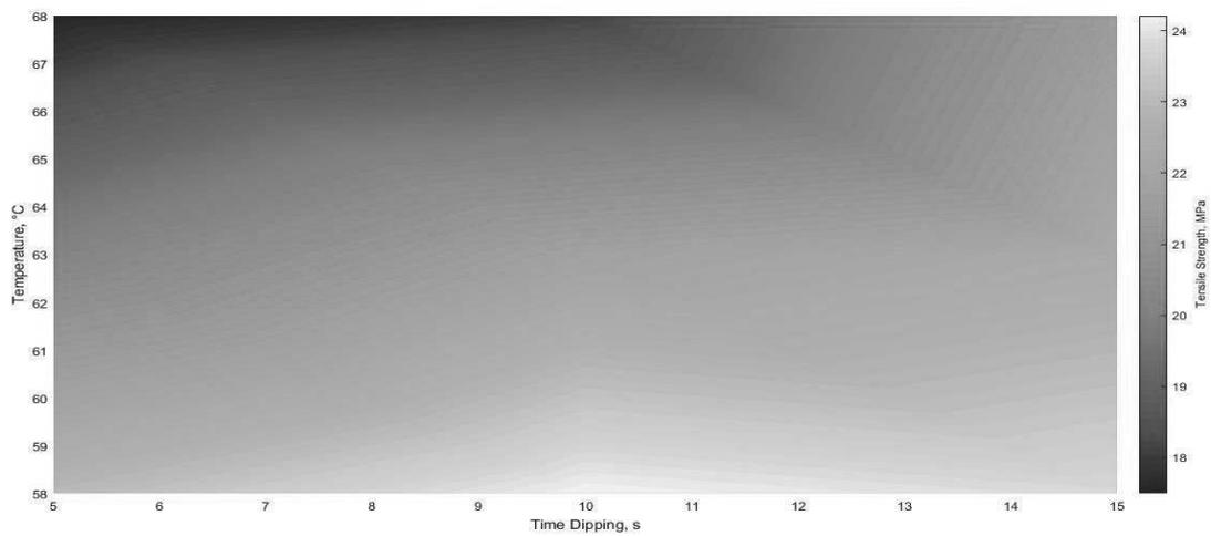
Figure 10: Contour of time and temperature against tensile strength of glove for 0.005 wt% of wetting agent
