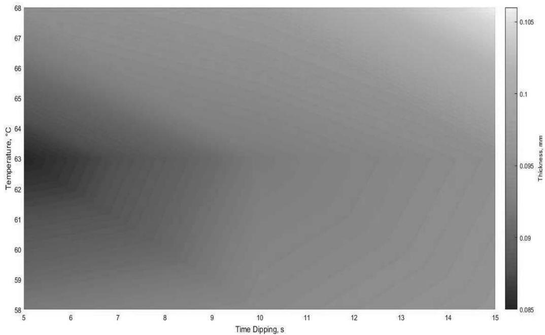
Figure 12: Contour of time and temperature against glove thickness for 0.03 wt% of wetting agent
