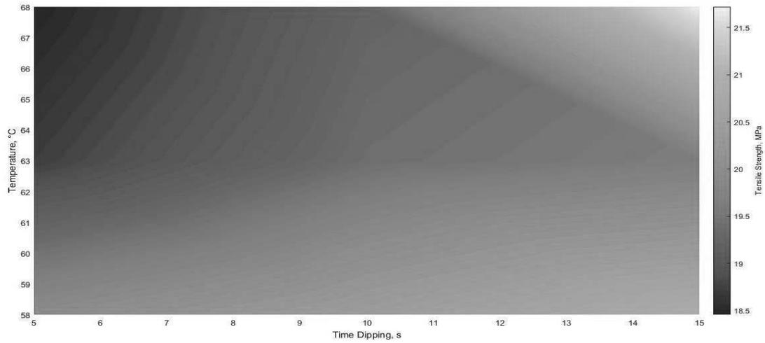
Figure 8: Contour of temperature and time against tensile strength of glove for 0.005 wt% of wetting agent
