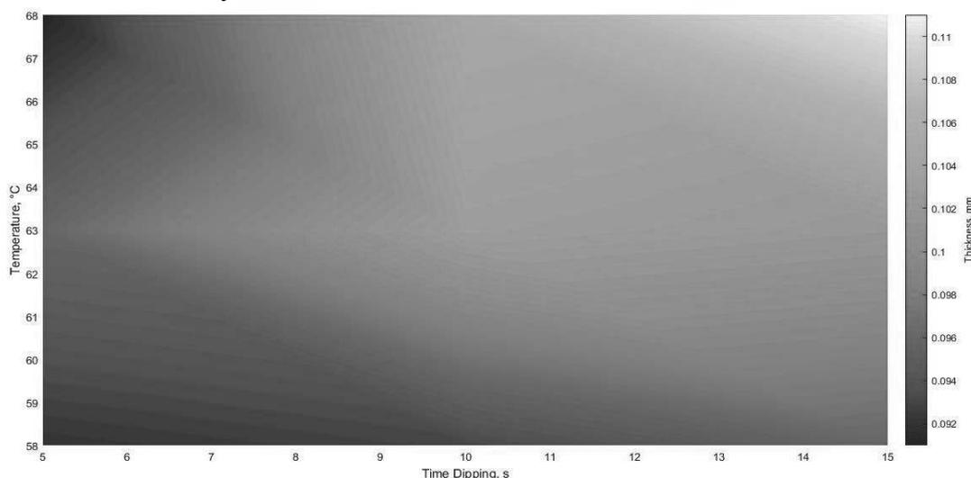
Figure 11: Contour of time and temperature against glove thickness for 0.005 wt% of wetting agent.
