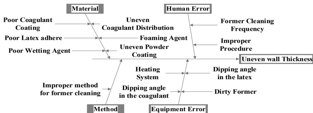
Figure 2: Ishikawa diagram for uneven thickness of glove [2-3].
