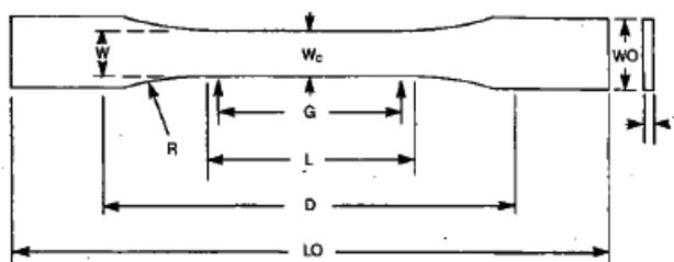
Figure 4: ASTM plate shape cutting [17].
