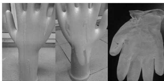
Figure 15: Foam on the mold (Left) and Latex uneven coating (Middle) and Sticky Glove at the cuff area (Right).
