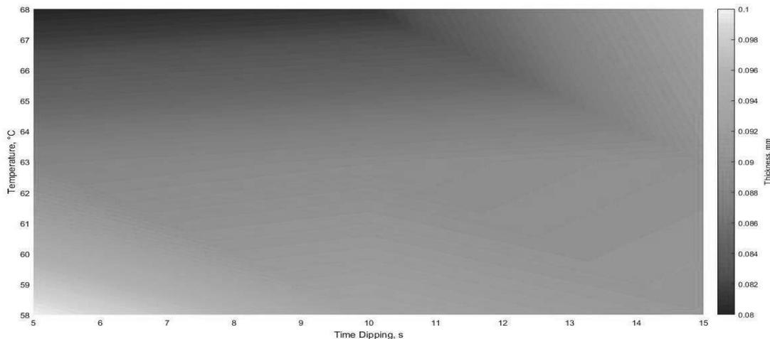
Figure 13: Contour of time and temperature against glove thickness for 0.05 wt% of wetting agent
