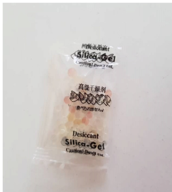
Fig. 4 Silica gel changed color after absorbed moisture.
