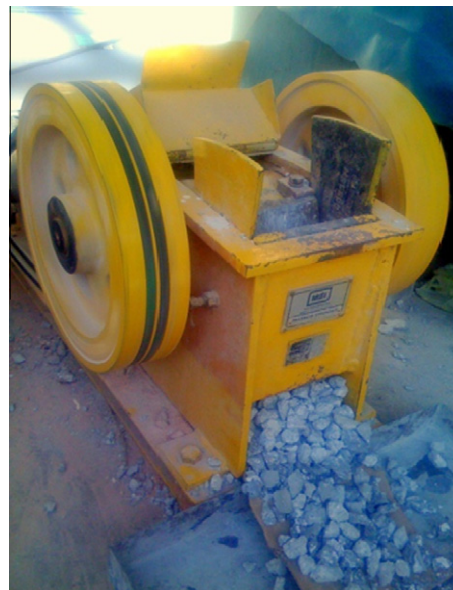
Fig. 1. Crushing process of RCA.
