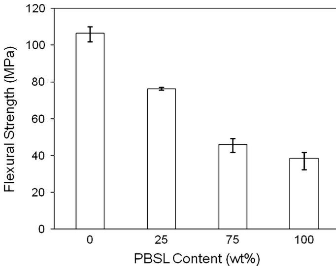
**Fig. 7** Influence of PBSL content on the flexural strength of PLLA blends
