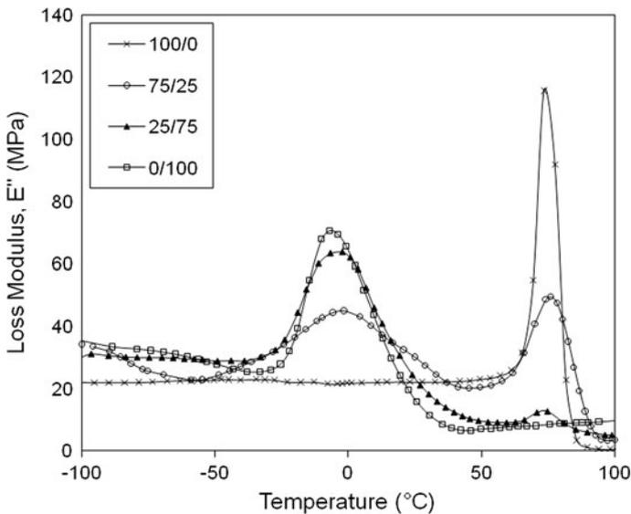
**Fig. 5** Temperature dependence of loss moduli ( $E''$ ) for neat PLLA, PBSL, and PLLA/PBSL blends
