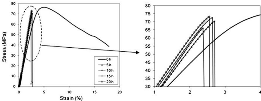
**Fig. 12** Flexural stress against strain curves of 75/25 PLLA/PBSL blend annealed for various time
