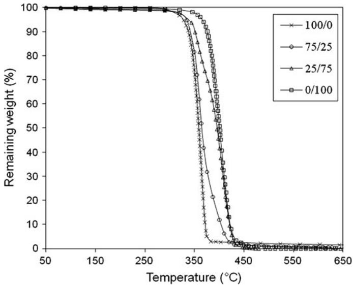
**Fig. 2** TGA curves of neat PLLA, PBSL, and PLLA/PBSL blends
