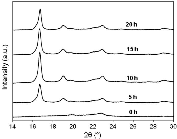
**Fig. 13** XRD patterns of 75/25 blend with different annealing time
