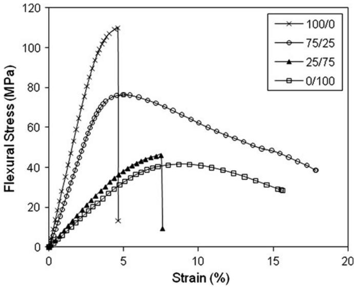
**Fig. 6** Plot of flexural stress against strain for PLLA/PBSL blends with various blending ratios
