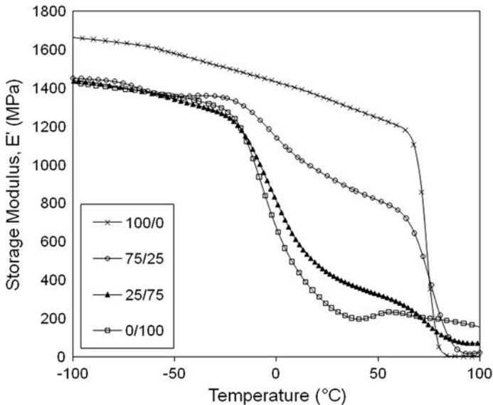
**Fig. 4** Storage modulus curves of neat PLLA, PBSL, and the blends
