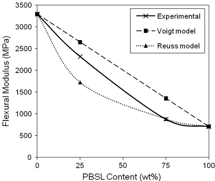
**Fig. 8** Change in flexural modulus of PLLA blends as a function of PBSL content
