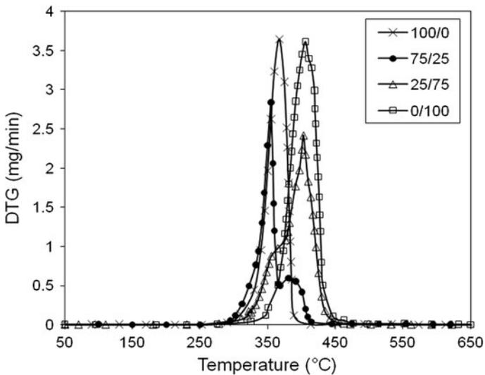
**Fig. 3** DTG curves of neat PLLA, PBSL, and PLLA/PBSL blends
