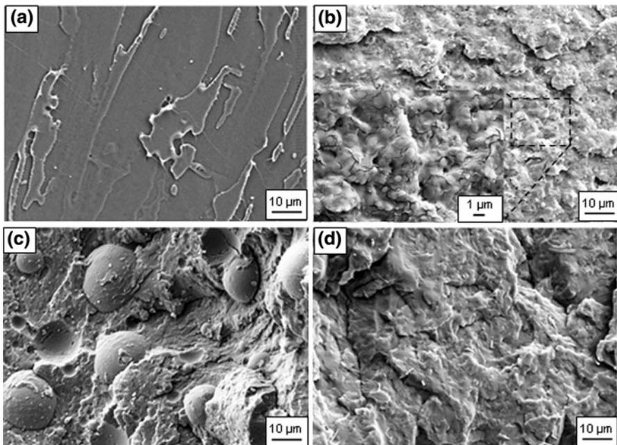
**Fig. 9** FESEM images showing the fracture surface of **a** neat PLLA, **b** 75/25 blend, **c** 25/75 blend, and **d** neat PBSL
