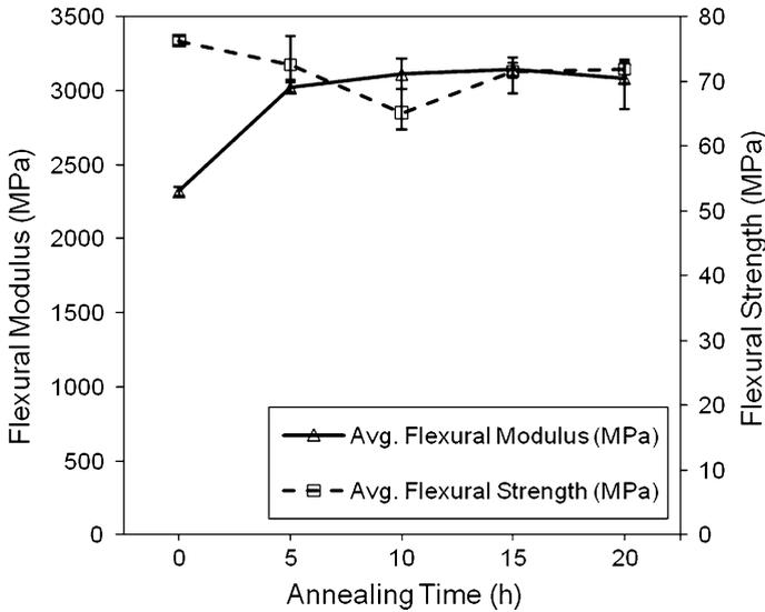
**Fig. 11** Changes in flexural modulus and strength of 75/25 blend as a function of annealing time
