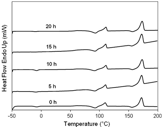
**Fig. 10** DSC thermograms of 75/25 blend annealed at 100 °C for various time periods
