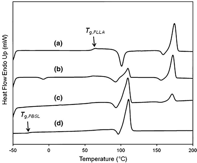
**Fig. 1** DSC thermograms of **a** neat PLLA, **b** 75/25 PLLA/PBSL blend, **c** 25/75 PLLA/PBSL blend, and **d** neat PBSL
