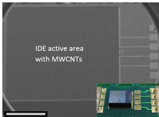
Fig. 3. IDE device with 1 \mu m width electrodes. Scale bar: 1 mm (Inset: Wire bonded device)
