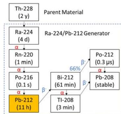
Fig. 3: Ra-224/Pb-212 generator (adapted from (41))
