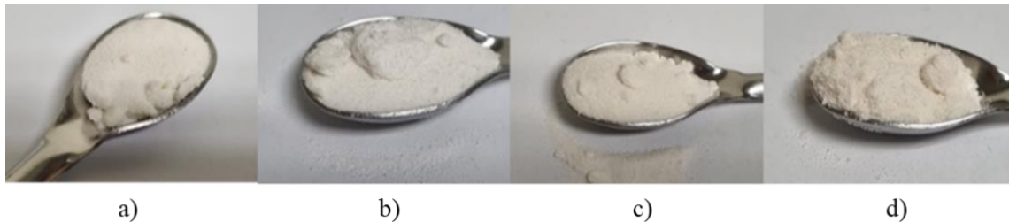
Figure 4. Sulfonated HIPS at a) 1 hour b) 2 hours c) 3 hours d) 6 hours.
