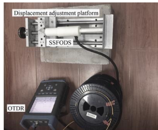
Fig. 13. Calibration test - designed SSFODS [64].
