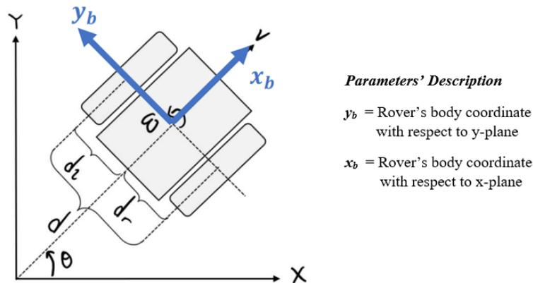
**Figure 5.** The redefined coordinate system (local frame) with respect to the global frame.
