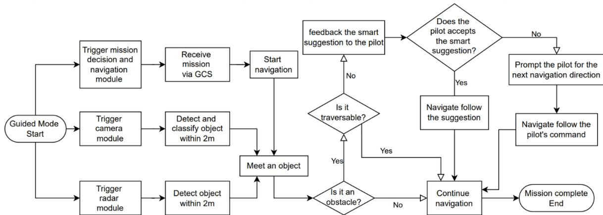
**Figure 2.** Flowchart of the level 3 autonomous rover operational system
