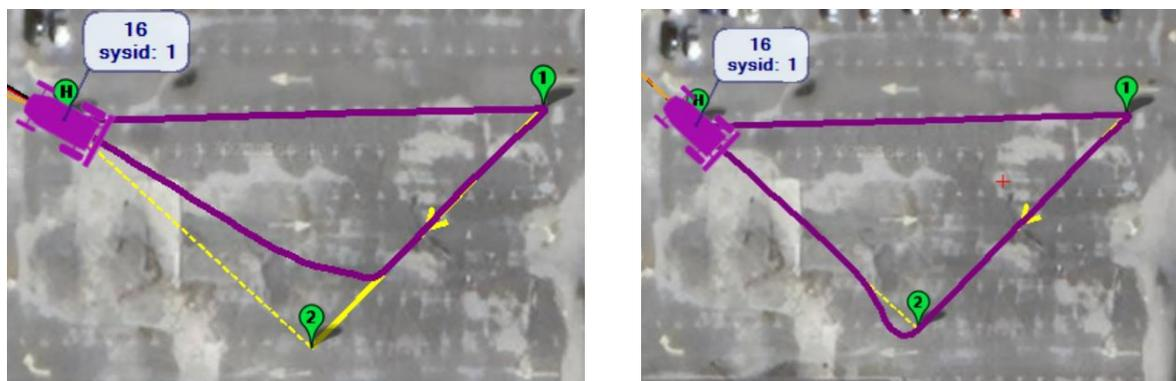
**Figure 12.** Rover's dynamic behaviour before (left) and after (right) PID tuning
