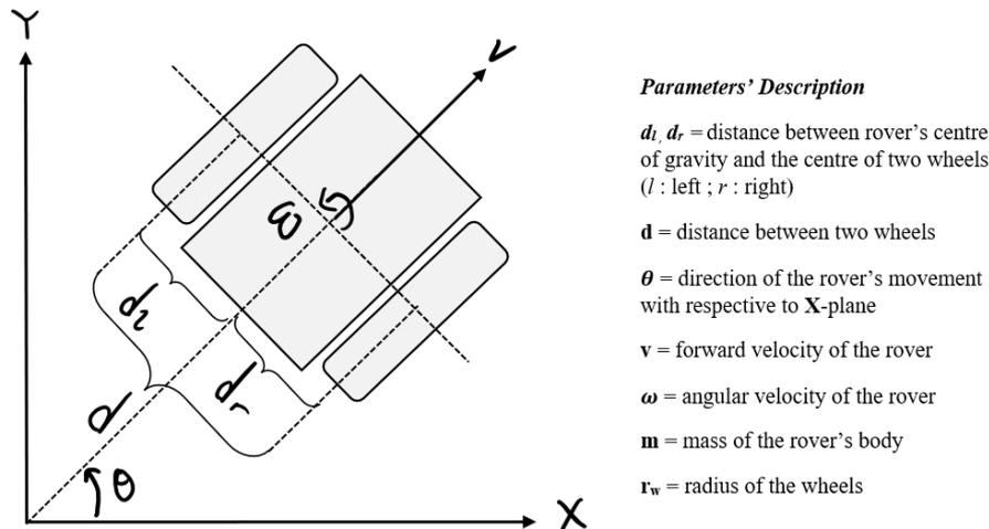
**Figure 4.** The dynamic model of the UGV and its parameters.
