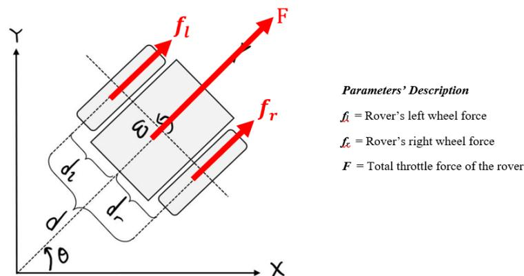
**Figure 6.** Force acting on rover's centre of gravity.
