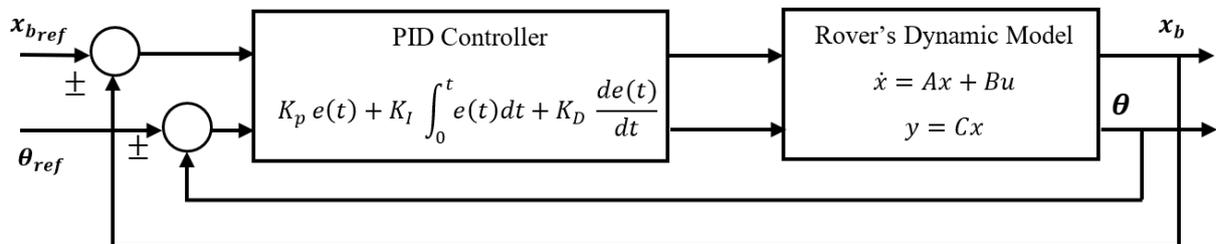
**Figure 7.** Closed-loop control system of the UGV
