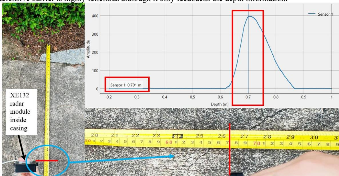
**Figure 10.** Radar accuracy testing on bushes
