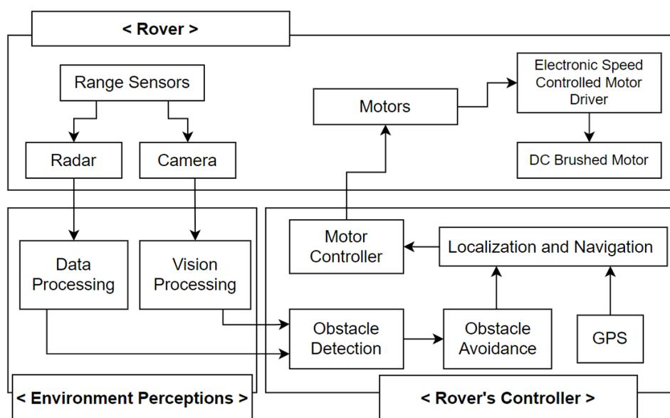
**Figure 1.** Block diagram of the autonomous rover integrated system
