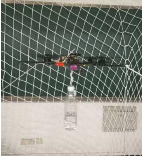
Fig. 7. Drone load disturbance test diagram
