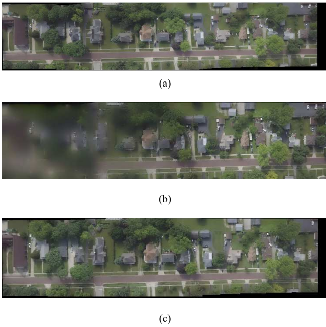
Fig. 6. (a) Results for the case of stitching all images at once; (b) stitching 20 images at a time from the front; and (c) stitching 20 images at a time and then further stitching the results in sets of 20.
