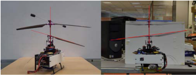
Fig. 9. Left: Maximum teetering angle of the lower rotor hub; Right: Maximum flapping angle of the lower rotor
