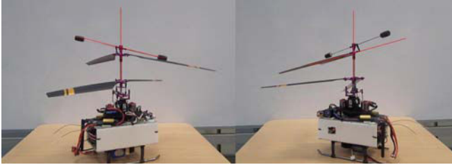
Fig. 10. Left: Maximum teetering angle of the stabilizer bar; Right: Maximum teetering angle of the upper rotor hub
