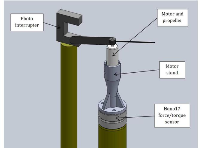
Fig. 5. Setup to obtain motor speed and thrust/torque produced
