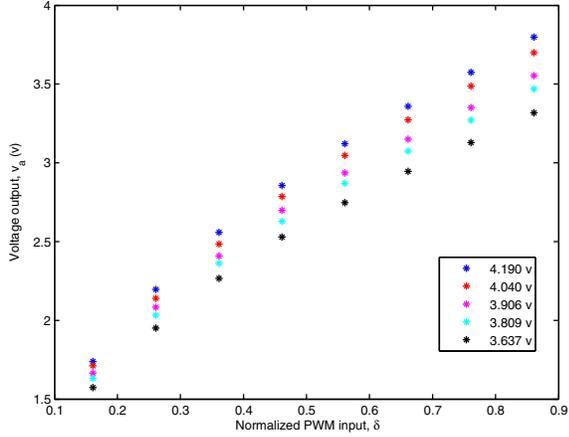
Fig. 2. Steady-state response of the ESC on two different inputs
