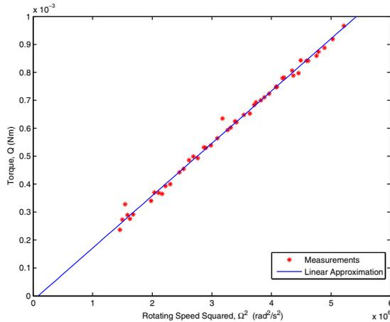
Fig. 7. Torque vs rotation speed squared
