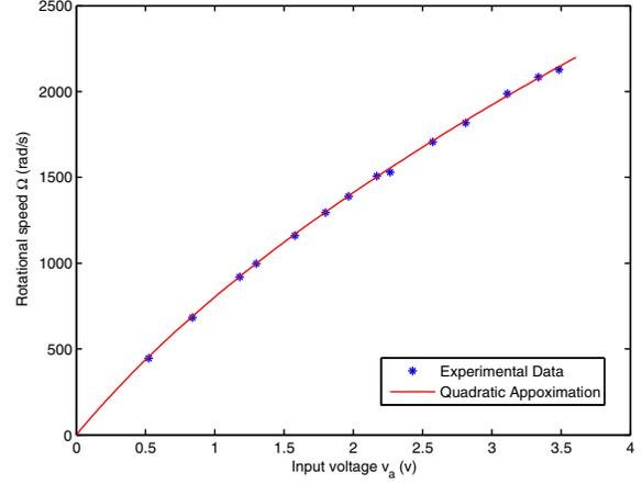
Fig. 4. Rotational speed response of the motor supplied with analog voltage
