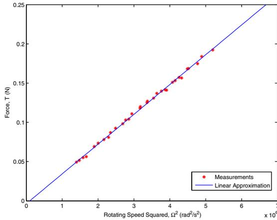
Fig. 6. Thrust vs rotation speed squared
