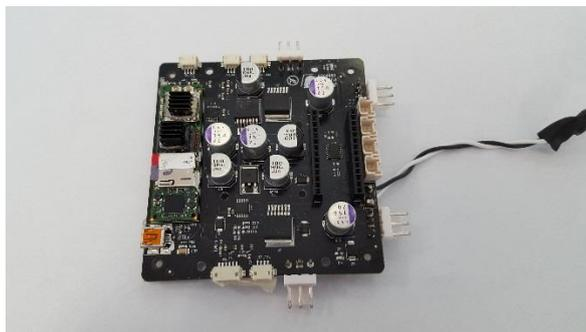
*Figure 3: Power Distribution Board*
