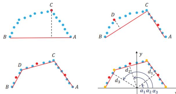
Figure 6: Split and Merge Algorithm to Extract Height
