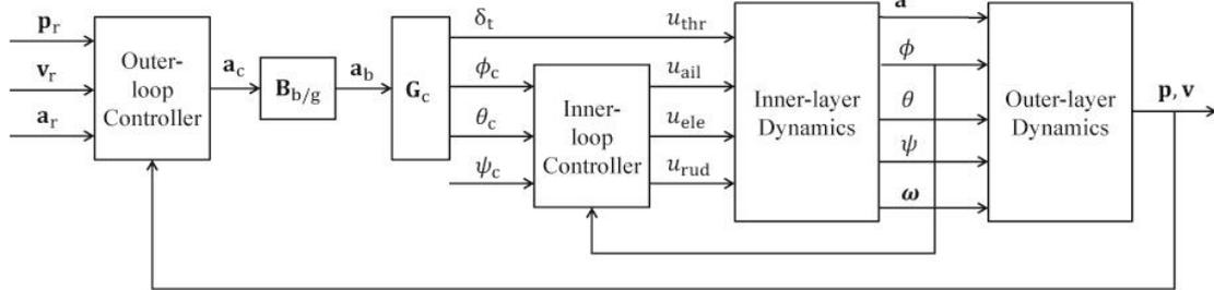
Figure 8: Controller Structure
