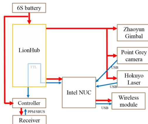
Figure 4: Hardware Structure of UAV
