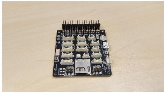
*Figure 2: Flight Controller*
