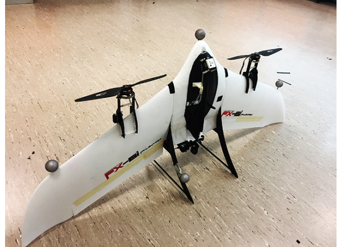
Fig. 1. KH-Lion, the tail-sitter hybrid UAV
