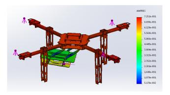
Figure 2: Mode shape of T-Lion at 39.9 Hz
