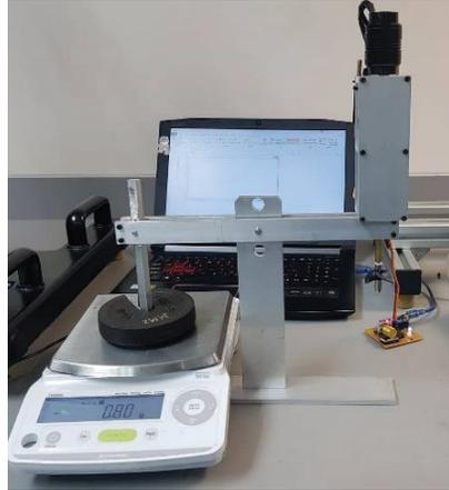
**FIGURE 4.** Experimental setup to identify the thrust produced from the motor and propeller.
