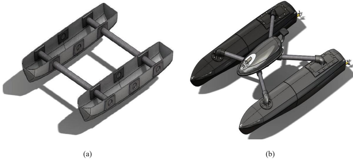
**FIGURE 2.** (a) First iteration of watercraft design. (b) Final iteration of the watercraft design.
