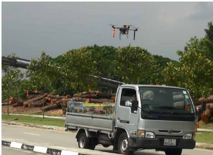
Fig. 16. Flight trials to autonomously track and land on a moving truck installed with the designed marker.
