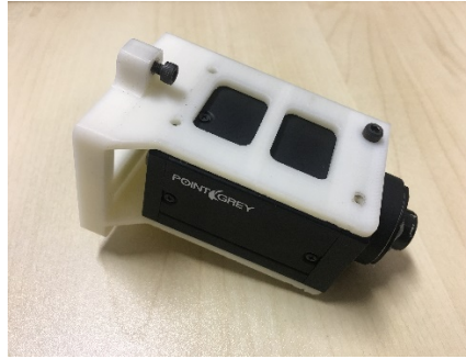
Fig. 4. Point Grey IR camera with a 3D printed adapter.
