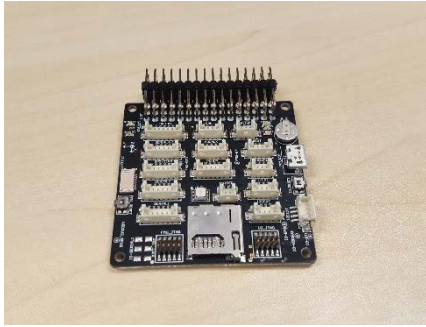
Fig. 3. Self-customized flight controller for T-Lion UAV.
