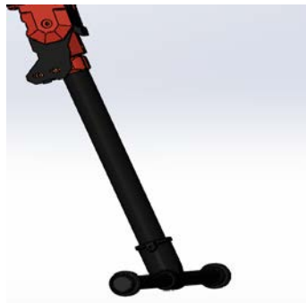
Fig. 14. Drone leg and landing gear (Combination of components from Figure 12a, 12b and 13a to 13c)
