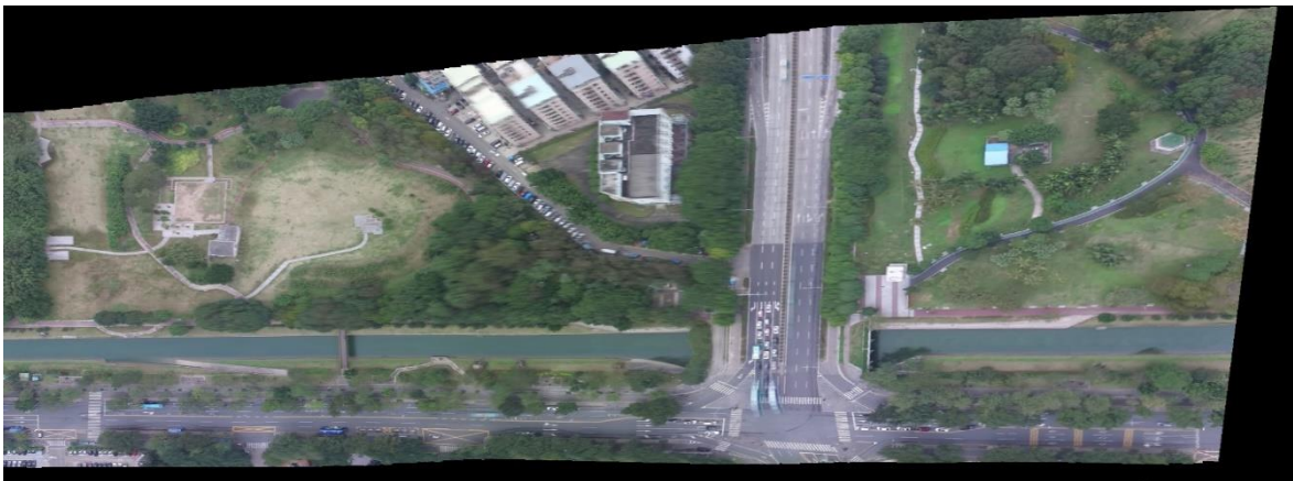
Figure 13. ORB Features-based with Improved RANSAC Algorithm to Stitch 100 Images
