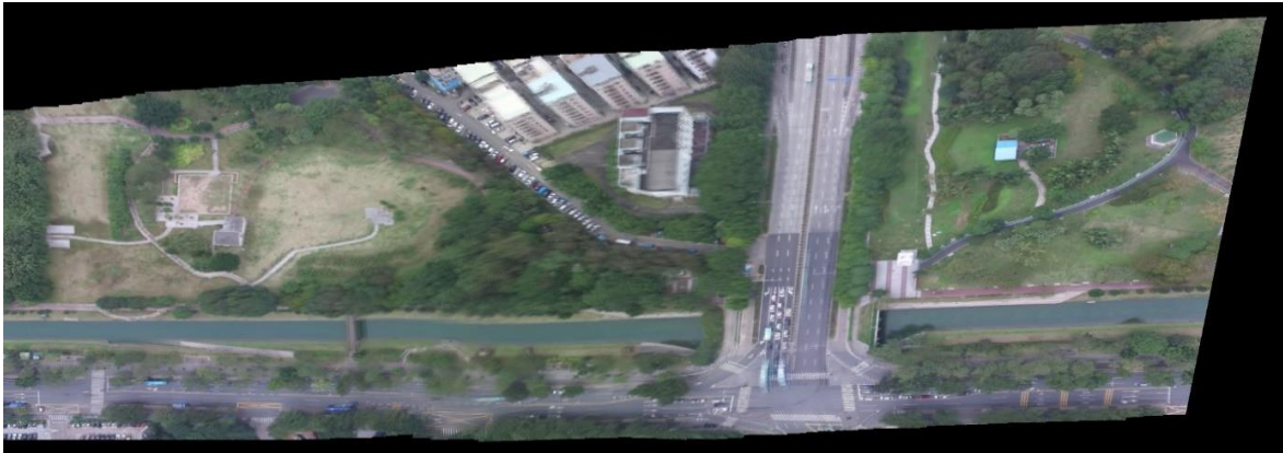
Figure 12. Original ORB Features-based Method to Stitch 100 Images
