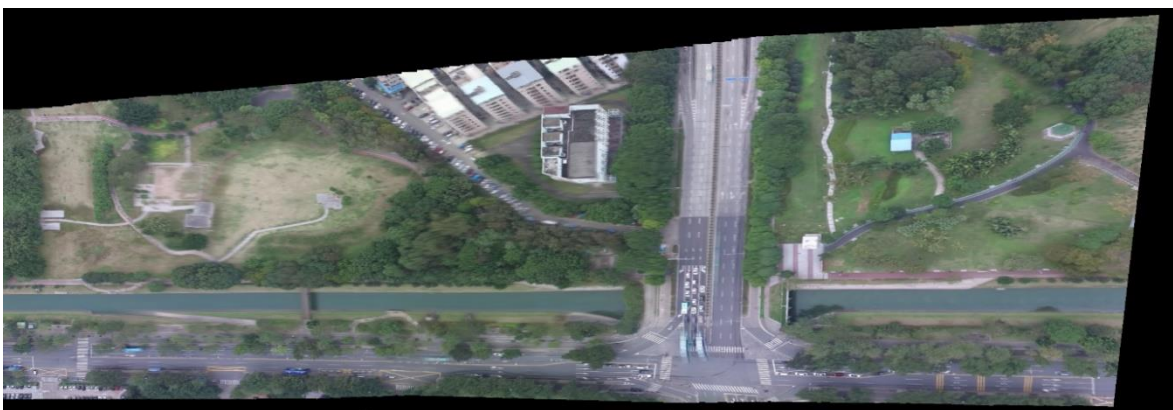
Figure 14. ORB Features-based with Improved RANSAC Algorithm and Improved Workflow to Stitch 100 Images
