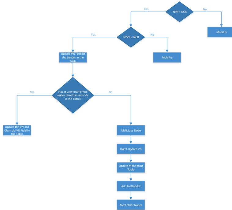
Figure 2. Protocol Model Flowchart, Phase Five.
