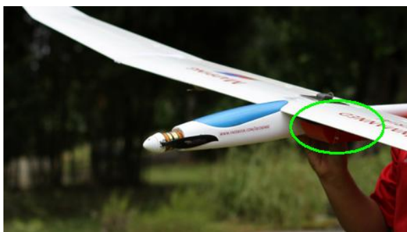
Figure 3: Payload (camera mount) beneath the CropCam UAV's wing (circled). Source : www.Geosense.com.my
