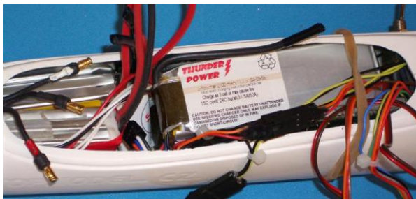
Figure 2: Cropcam UAV with small payload compartment. Source : www.topmodelcz.cz
